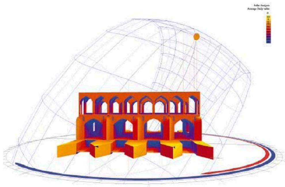
Figure 7. Solar analyses displaying the shaded area of the two floors of Khaju Bridge (photograph by Hensel, Gharleghi, 2012).
