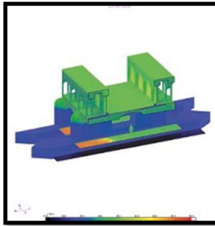
Figure 5. Picture A shows an axonometric of the bridge and Picture B shows the section of Khaju Bridge. Analyses of heat transfer shows that surface temperature of Khaju Bridge during the summer time is cool owing to the fact that the special design of the structure brings about a comfortable environment on this bridge. (Hensel, Gharleghi, Craig, Hensel, 2012) (photograph by Hensel, Gharleghi, Craig, Hensel, 2012).
