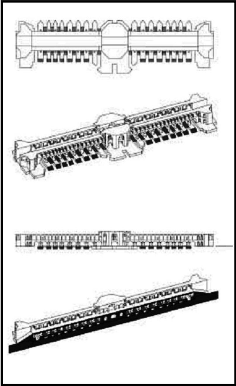
Figure 4. Plan, axonometric, elevation and axonometric sections of the Khaju Bridge in Isfahan (photograph by Michael, Gharleghi, 2012).
