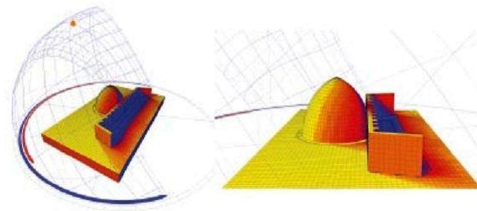
Figure 6. 3D models of Khaju Bridge with solar analyses, the facade of Khaju Bridge protects the water pond from the deleterious effects of the sun and wind. Research shows that during the winter time the pond does not receive any direct sunlight which can mean ice forming in cooler temperatures above 0°C. (Hensel, Gharleghi, Craig, Hensel, 2012) (photograph by Hensel, Gharleghi, Craig, Hensel, 2012).
