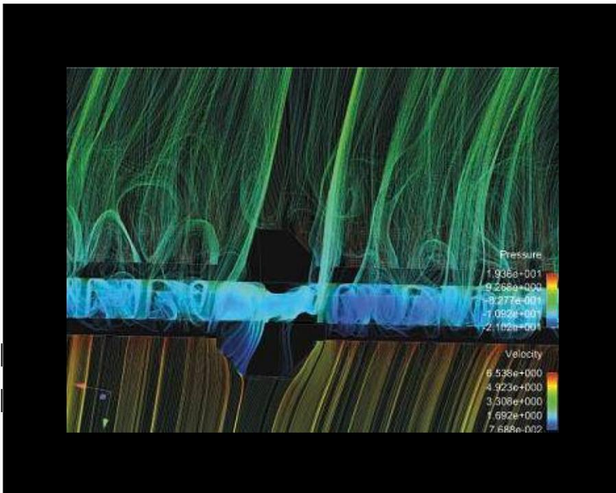
Figure 11. Analysis showing that the evenly spaced arches in this structure change the wind speed bringing a low breeze (3.2 kilometres per second) onto the roadway. This means that the structure brings about a comfortable environment along the path (Hensel, Gharleghi, Craig, Hensel, 2012) (photograph by Hensel, Gharleghi, \_Craig, Hensel, 2012).
