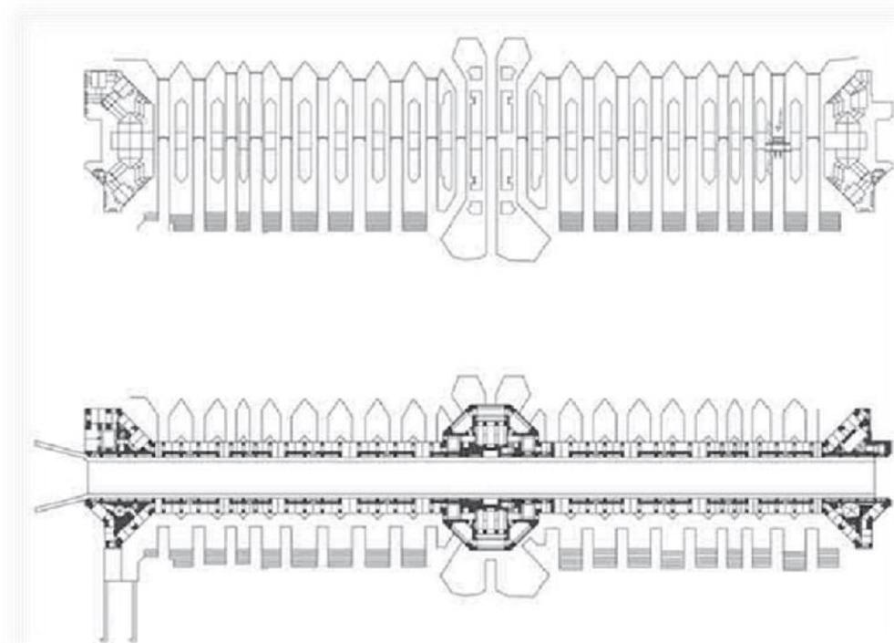
Figure 15. The top plan presents a base balance and channels of Khaju Bridge which are made from rock and the down plan presents the level crossing of the bridge (photograph by Shah Karami, 2006).
